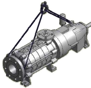
Fig. 5: lifting the pump
