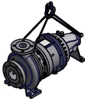
Fig. 4: Transporting the pump
