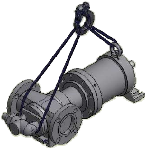
Fig. 6: lifting the pump
